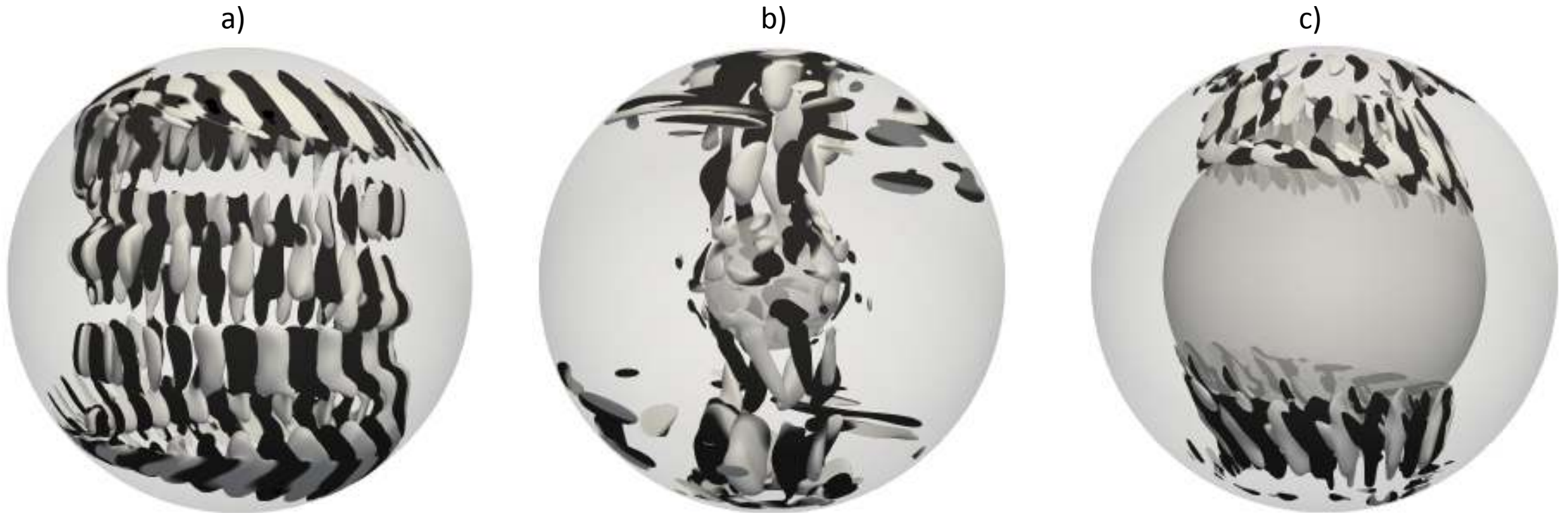
Isosurfaces of the anti-symmetric energy in the mean fluid rotating frame for (a) \eta = 0.01 , Po = 8 \times 10^{-3} (b) \eta = 0.3 , Po = 8 \times 10^{-3} and (c) \eta = 0.7 , Po = 8.5 \times 10^{-3} . In each case \alpha = 120^\circ and E = 3.0 \times 10^{-5} . Color correspond to positive (black) and negative (white) axial velocity. The snapshots are taken during the initial growth phase of the instability.
